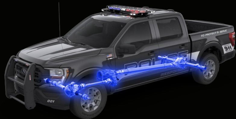
TORQUE-ON-DEMAND® 4x4 TRANSFER CASE
