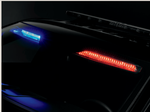
Front Interior Visor Light Bar (96W). Includes (2) backlit flashing, linear high-intensity LED lights (driver side red; passenger side blue) mounted inside the windshield glass. Lights can be programmed for tricolor (red, white, blue) patterns.
