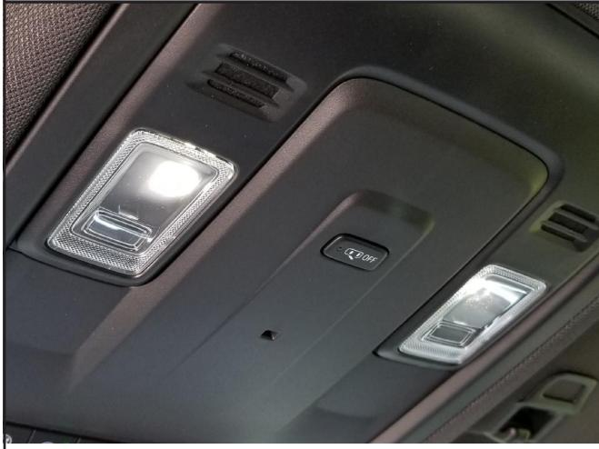
There are dome lamps in the overhead console and the headliner. To change the dome lamp settings, activate the following:
