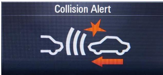
The Forward Collision Alert (FCA) system may help to avoid or reduce the harm caused by front-end crashes with vehicle being followed. When approaching a vehicle ahead too quickly, FCA provides a red flashing alert on the windshield and rapidly beeps. FCA also lights an amber visual alert if following another vehicle much too closely. FCA detects vehicles within a distance of approximately 60m (197 ft) and operates at speeds above 8 km/h (5 mph).
