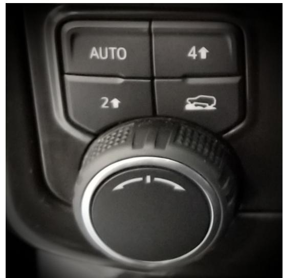
TRANSFER CASE - Autotrac with AUTO 4WD, 4HI or 2HI electronic settings (includes Terrain Mode). Single-speed, electronic transfer case does not include neutral and cannot be dinghy towed.
