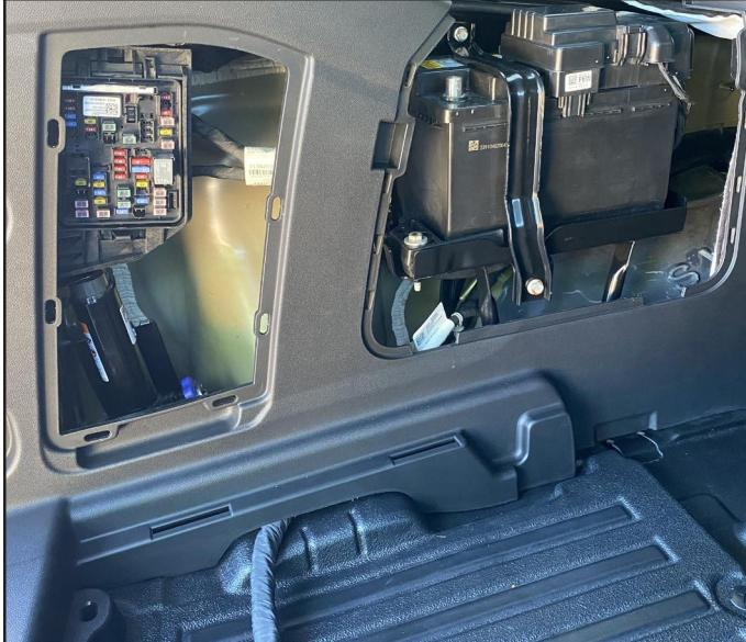
The auxiliary battery negative battery cable is disconnected during shipment. It must be connected by the customer for proper operation of blunt cut battery feed circuits and auxiliary battery charging system
