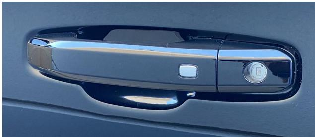
The remote key must be within 3 ft (1 m) of the liftgate or door being opened or locked. Press the button on the door handle to open.
