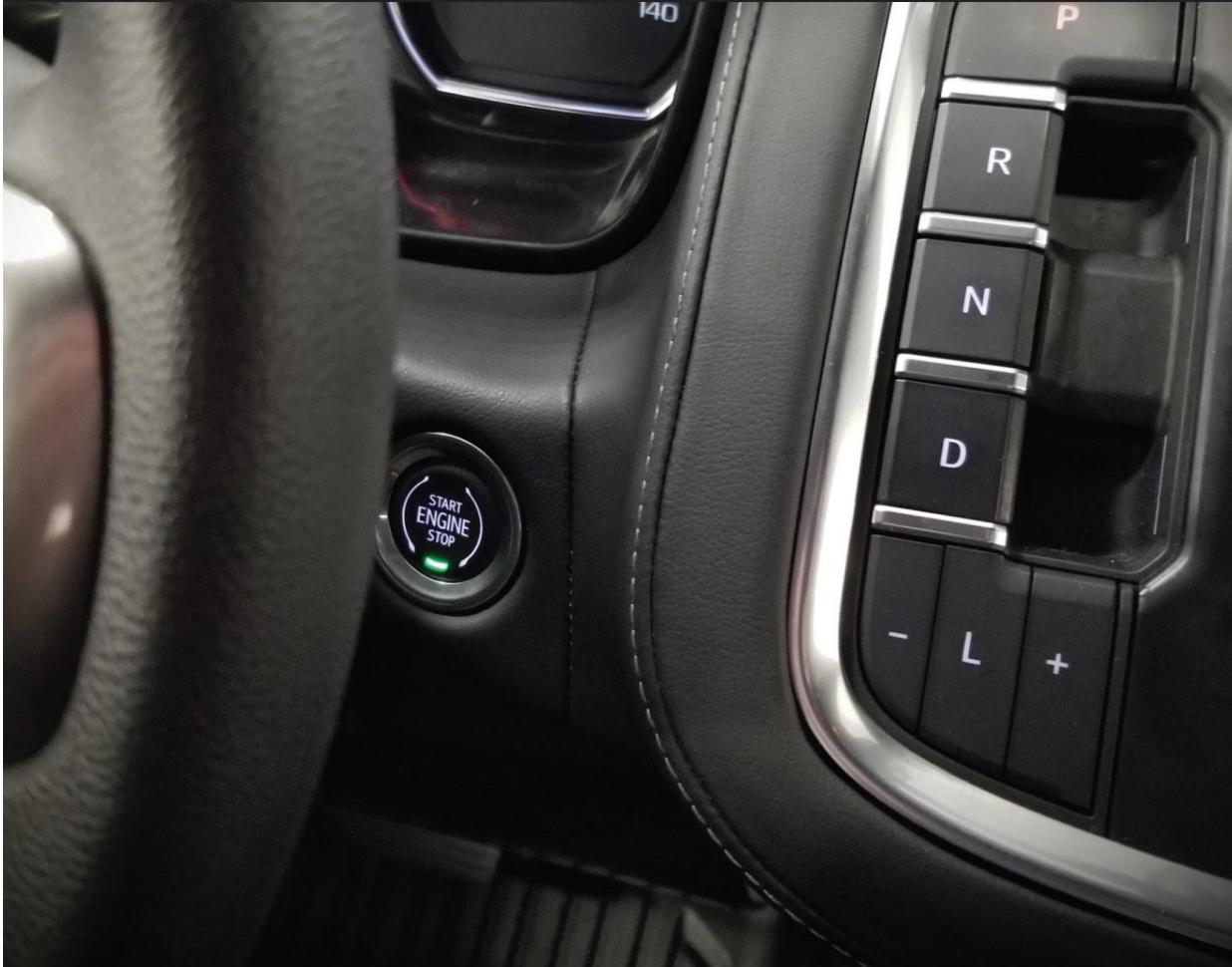
This vehicle is equipped with an electronic transmission with controls mounted next to the instrument panel for easy access. The shift switches are designed to prevent inadvertent shifting out of P (Park) unless the ignition is on and the brake pedal is applied. Push-to-shift transmission technology is intuitive to use, with pull switches for Drive (D) and Reverse (R) and push switches for Park (P), Neutral (N) and Low (L).
