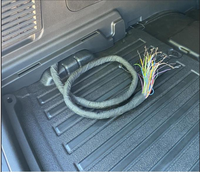
Cargo area branch with circuits for customer connection<sup>1</sup>. Tagged circuits listed in UPFIT WIRING HARNESS CIRCUIT LIST
