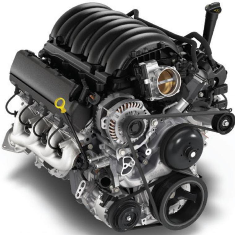
Dynamic Fuel Management allows engine to operate in 17 different cylinder patterns (as few as two cylinders) to optimize power delivery and efficiency. The DFM controller calculates 80 times per second to determine how many cylinders are required to meet the driver's requested torque.
