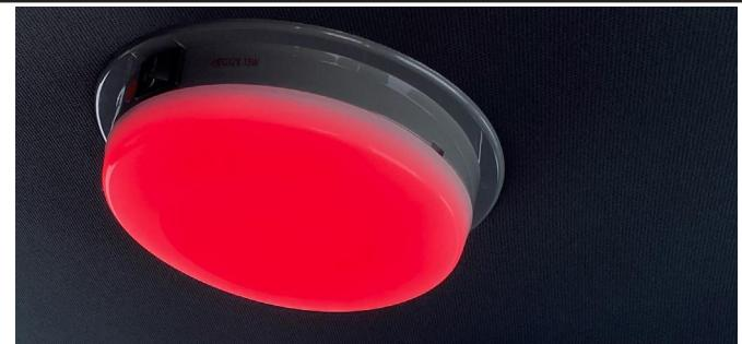
Auxiliary dome lamp is located on the headliner to the rear of the overhead console and is switched at the rear lamp base. Lamp is wired separately standard dome lamps with red and white LED bulbs.
