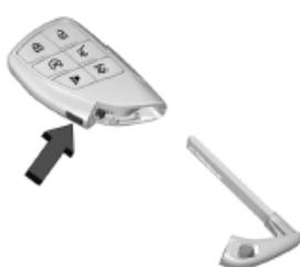
The mechanical key inside the remote key is used for the driver door, glove box and spare tire access.
