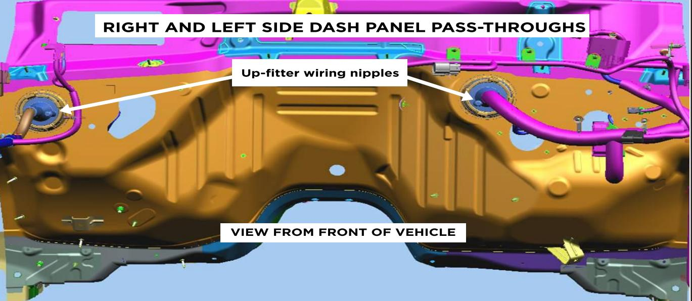
Provides pass throughs for a small number of wires and are located at the left and right sides of the front of dash. Carefully remove or puncture only the nipple portion for the passage of upfitter wires and silicone seal around the wire after installation. Note that a vehicle harness is passing through the grommets and care must be taken to avoid damaging these harnesses especially in the instrument panel interior.
