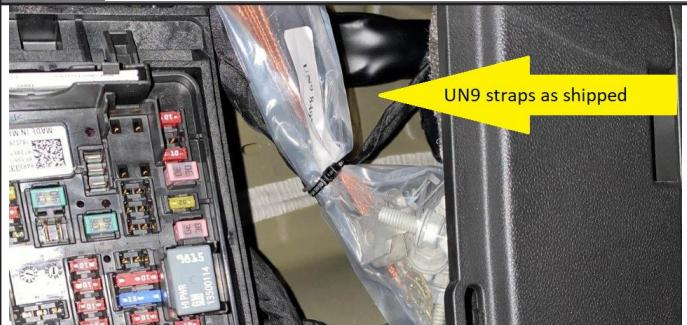
The UN9 ground straps and hardware kit is shown below in the plastic bag which is wire tied to the rear cargo blunt cut harness and accessible when the driver side rear cargo area fuse panel access door is removed. This kit should be installed per the I-sheet which can be found at the GM Upfitter.com site at the following link: [https://www.gmupfitter.com/files/media/photo/1500/UI%20Bulletin\\_173\\_PRELIM.pdf](https://www.gmupfitter.com/files/media/photo/1500/UI%20Bulletin_173_PRELIM.pdf)
