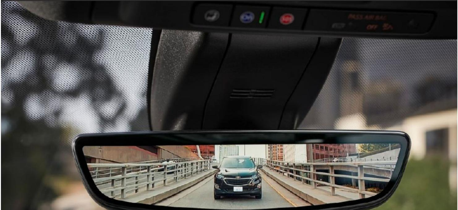
Inside rearview auto-dimming with full camera display. Includes (CWA) Rear Camera Mirror Washer. Not available with (PQA) Safety Package
