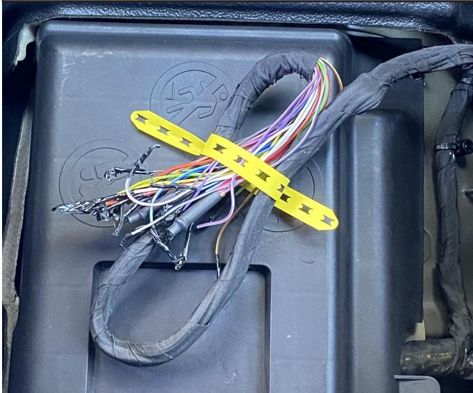
Front Center area upfitter branch harness<sup>1</sup> with tagged circuits for customer connection. View with center front seat removed per Option 5Y1. Branch is forward of seat without Option 5Y1. Tagged circuits are listed in UPFIT WIRING HARNESS CIRCUIT LIST.
