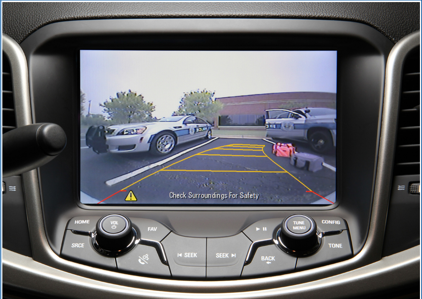
8-inch backup display with steering path guides displayed in radio screen.
